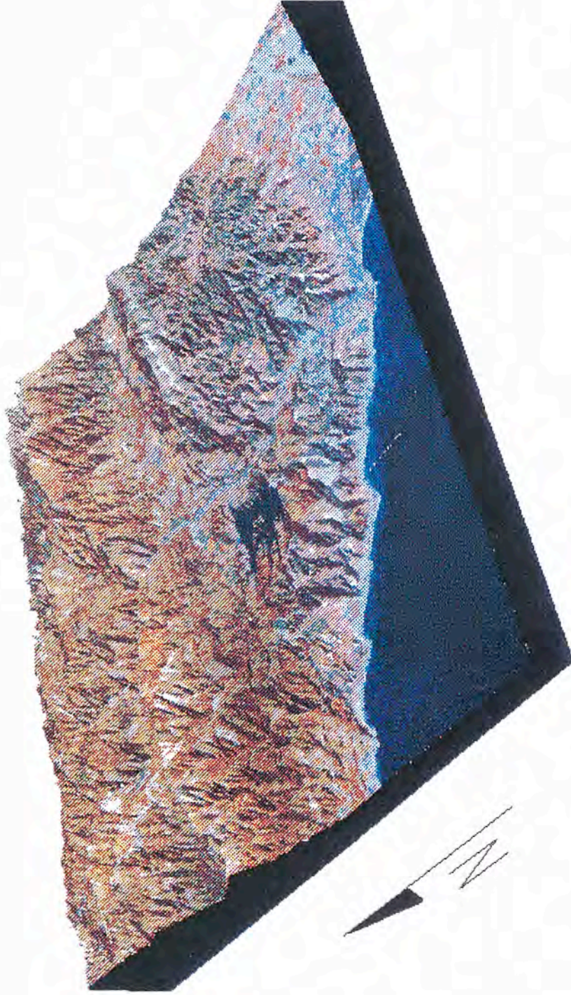
Fig. X-2. VENTURA RIVER WATERSHED THREE-DIMENSIONAL RELIEF MAP. View from the Pacific Ocean northward into Ventura River system. Processed image is a false-color-infrared composite (Landsat MSS Bands 7,5, and 4 rendered as red, green, and blue, respectively) for December 17, 1982. The Landsat image has been draped over a digital elevation model for the basin. Exaggerated vertical elevation emphasizes the rapid rise of the terrain from sea level to over 1800 m. The relatively flat area in the east-central part of the basin is the Ojai Valley.
